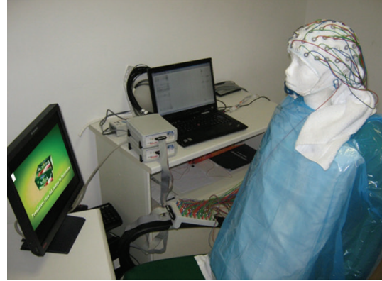
FIGURE 1: Experimental setup employed for the simulated electrical recording on a mannequin head by means of a 61-channel EEG cap. The polystyrene mannequin head was posed in front of a screen to include the interferences on signals due to the presence of a monitor.
