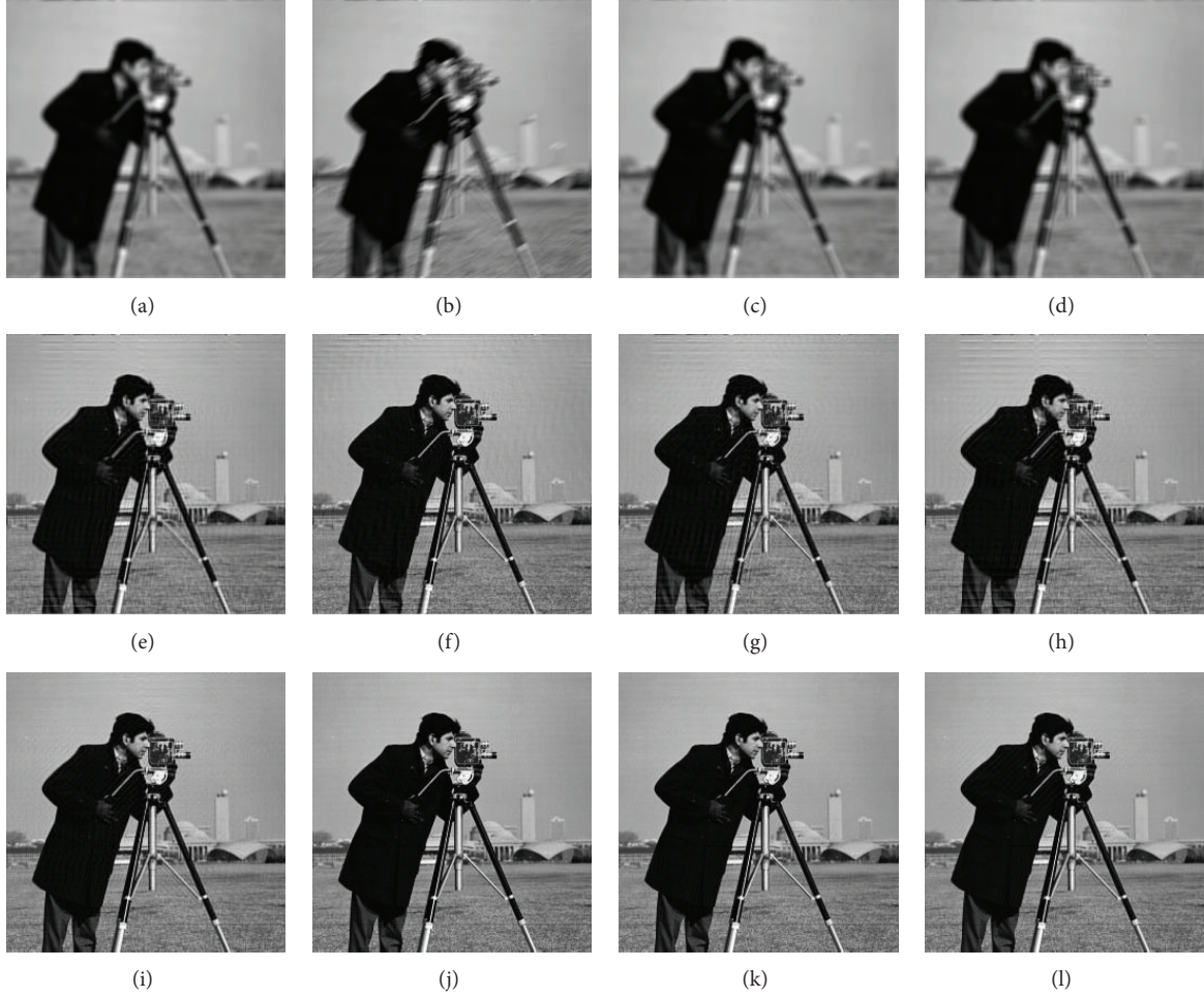
FIGURE 2: Deblurring of “Cameraman.” (a)–(d) Gaussian blurred image, linear motion blurred image, out-of-focus blurred image and uniform blurred image, respectively. (e)–(h) Images deblurred by SBI. (i)–(l) Images deblurred by PSBI.
