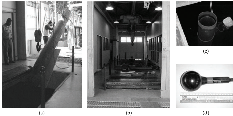
Figure 16: Photos of the experiment: (a) tube installation through the water tank input gate; (b) tank facilities; (c) tube inside the tank (view through the gate); (d) acoustic transducer ITC 1032 (source/receptor).
