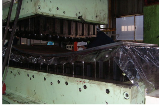
Figure 1: An apparatus of multiple-point press machine used for thick plate forming.
