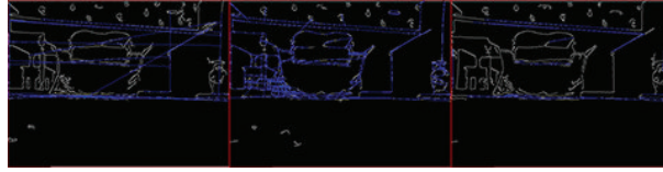
Figure 2: Comparison of Hough line parameters. Left image large maximum pixel gap value, middle image low line votes, and segment length value, right image optimal found settings.
