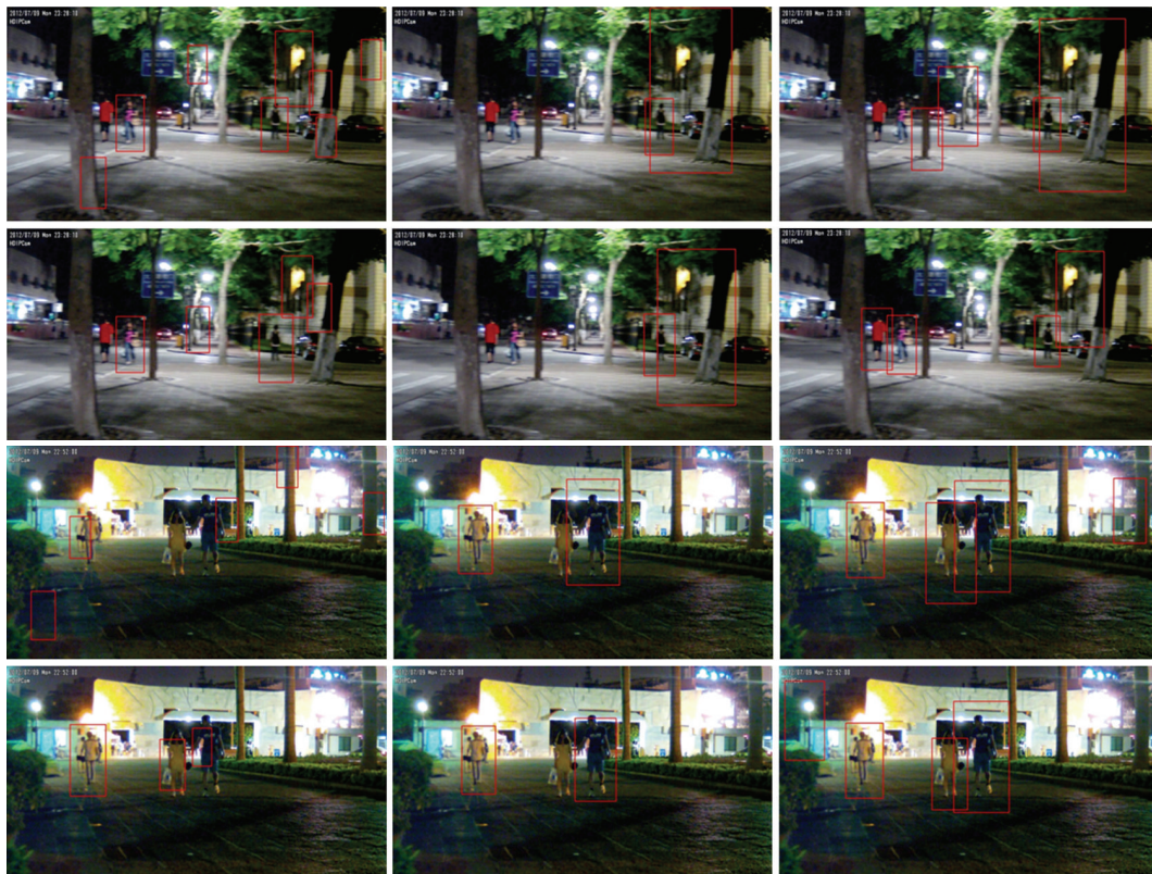
FIGURE 10: Detection results on XMU-NIR. From left to right and top to down, the classifiers are HOG_lin, LBP_lin, HOG.LBP_lin, HOG_HIK, LBP_HIK, and HOG.LBP_HIK.
