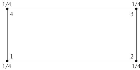
Figure 6.1. Basic rectangle with only four points. Point numbers are inside, weight fractions are outside.
