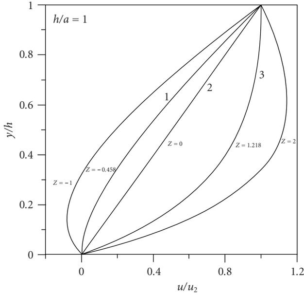
FIGURE 3.1. Velocity profiles for Couette flow with Lorentz force for  $h/a = 1$  and different values of the Chandrasekhar number. The case  $Z = 0$  corresponds to Couette flow with upper plate moving.
