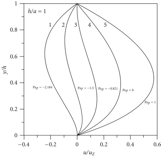
FIGURE 3.3. Velocity profiles for Poiseuille flow with Lorentz force for  $h/a = 1$  and different values of the  $Pa_p$  parameter. The case  $Pa_p = 0$  corresponds to zero pressure gradient.
