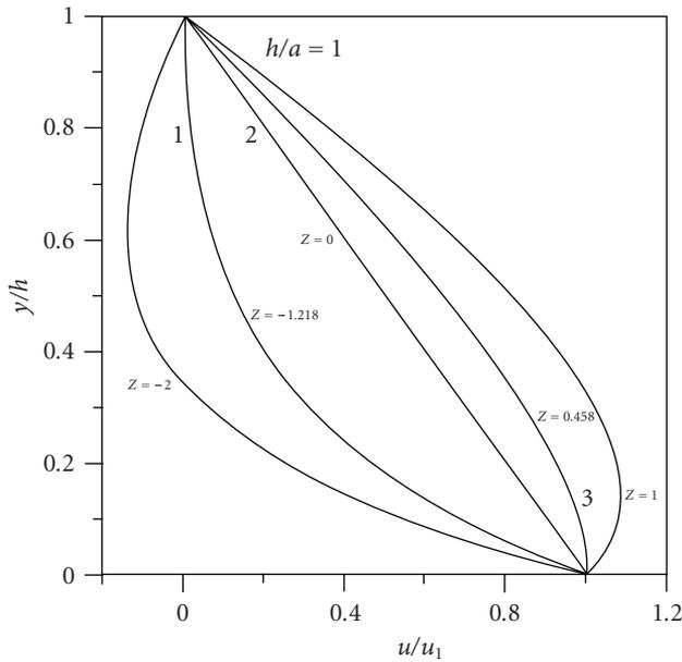
FIGURE 3.2. Velocity profiles for Couette flow with Lorentz force for  $h/a = 1$  and different values of the Chandrasekhar number. The case  $Z = 0$  corresponds to Couette flow with lower plate moving.
