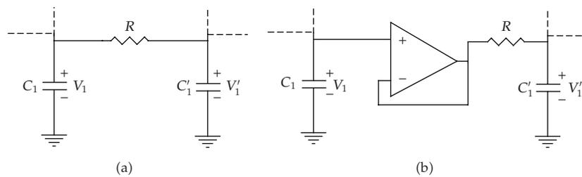
**Figure 10:** Coupling schemes: (a) bidirectional; (b) unidirectional.
