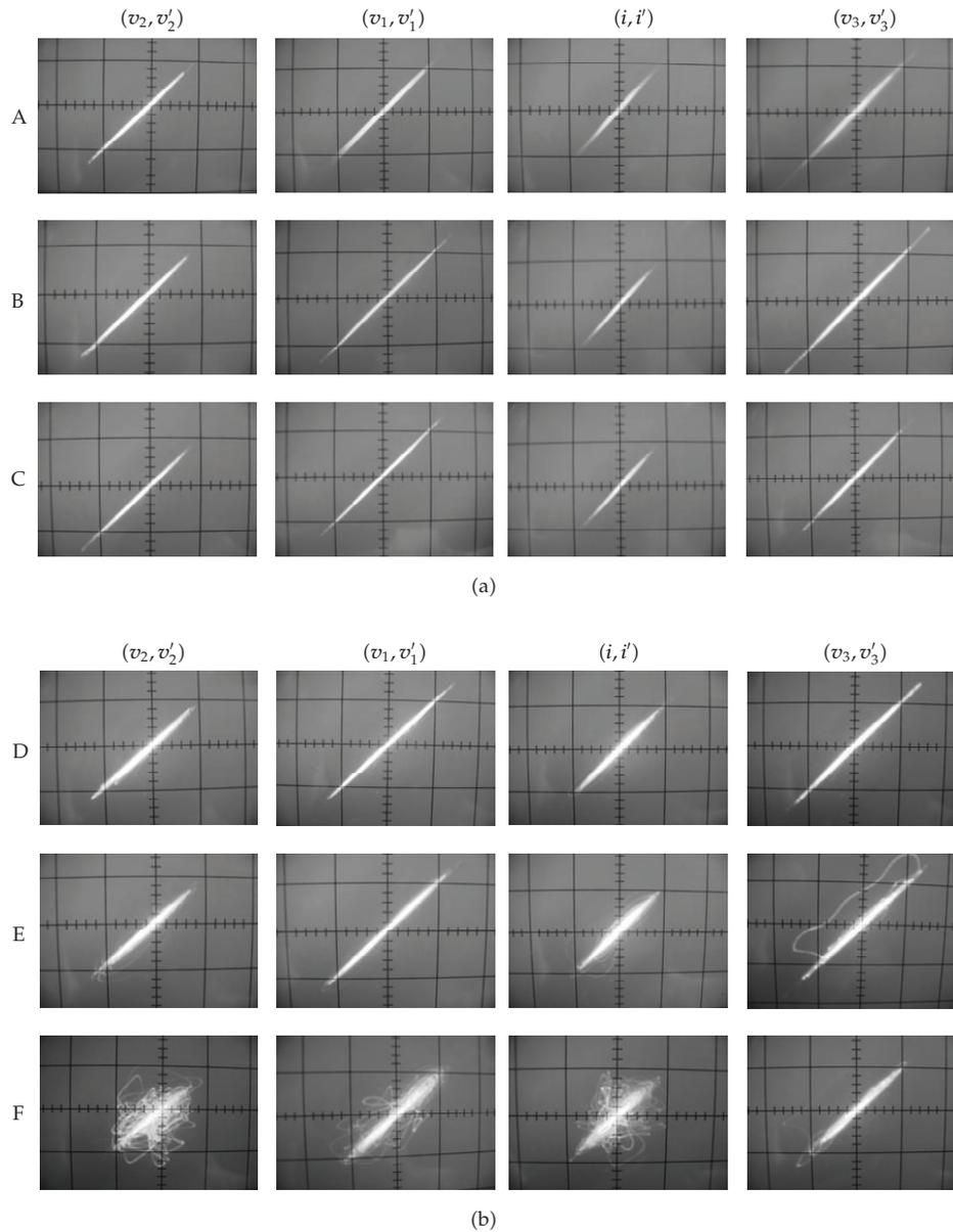
**Figure 11:** (a) Experimental trajectories near the synchronization hyperplane for several values of the unidirectional coupling resistor. A:  $0\ \Omega$ ; B:  $100\ \Omega$ ; C:  $220\ \Omega$ . (b) Continuation of Figure 11(a). D:  $470\ \Omega$ ; E:  $1.0\ \text{k}\Omega$ ; F:  $2.2\ \text{k}\Omega$ .
