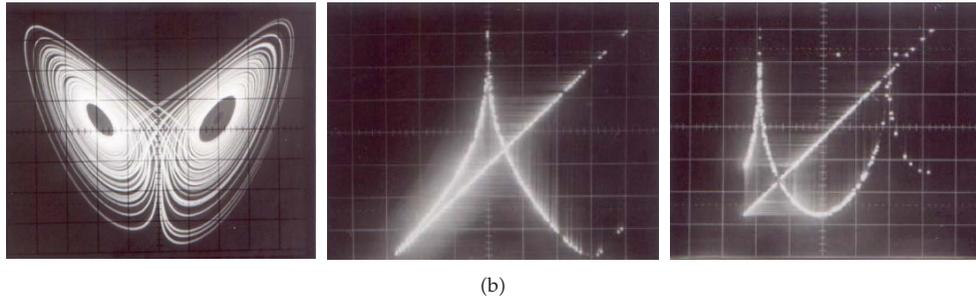
**Figure 7:** (a) Simplest circuit for the 3D standard Lorenz equations. (b) Experimental results from the circuit of Figure 7(a): butterfly attractor on the plane  $v_1 \times v_2$ ; Lorenz maps showing single and double cusps  $v_2(t_n) \times v_2(t_{n+1})$ . The straight line in each picture is given by  $v_2(t_{n+1}) = v_2(t_n)$ .  $L = 10$  mH,  $C_1 = 22$  nF,  $C_2 = 1$  nF,  $R_1 = 1.5$  k $\Omega$ ,  $R_2 = 100$   $\Omega$ ,  $R_3 = 160$  k $\Omega$ ,  $R_4 = 1$  k $\Omega$ .
