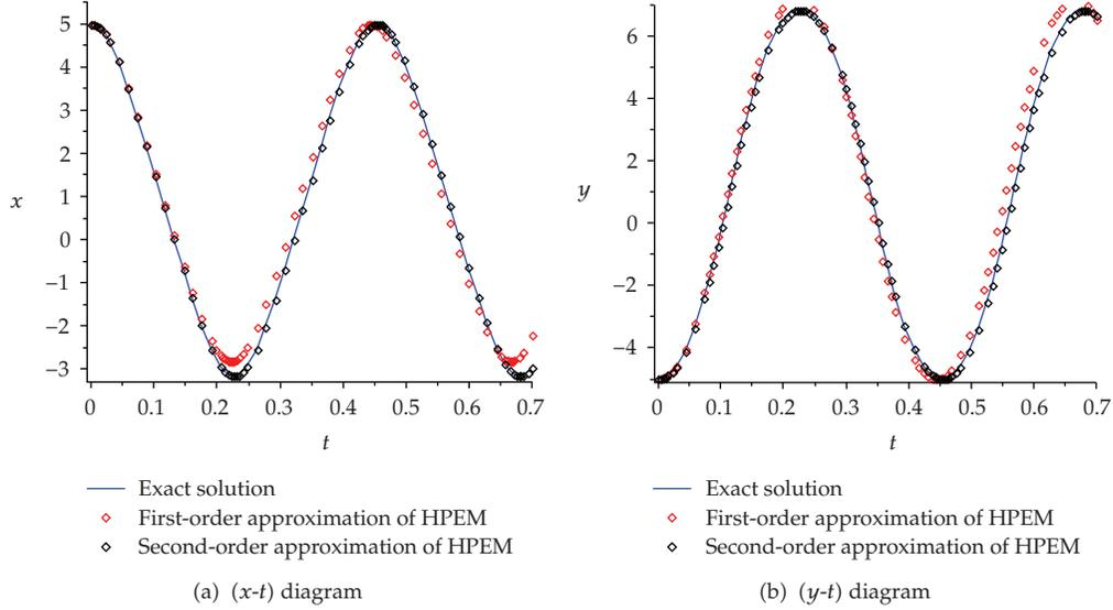
**Figure 10:** Comparison of the first- and second-order analytical approximate solutions with the exact solution for  $m_1 = 3.0, m_2 = 5.0, k_1 = 2.0, k_2 = 5.0$  with  $x(0) = 5.0$  and  $y(0) = -5.0$  (Case 3).
