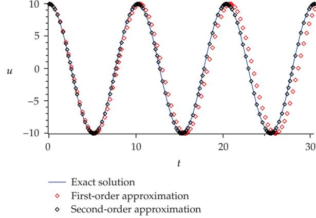
**Figure 5:** Comparison of approximate periodic solutions of Buckling of a Column equation (Case 1) with the exact one for  $m = l = P = k_1 = 10.0$ , and  $k_3 = 50.0$  with  $u(0) = 10.0$ .
