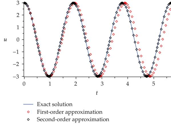
**Figure 4:** Comparison of approximate periodic solutions of Buckling of a Column equation (Case 1) with the exact one for  $m = 1.0$ ,  $l = 1.5$ ,  $P = 5.0$ ,  $k_1 = 5.0$ , and  $k_3 = 6.0$  with  $u(0) = 3.0$ .
