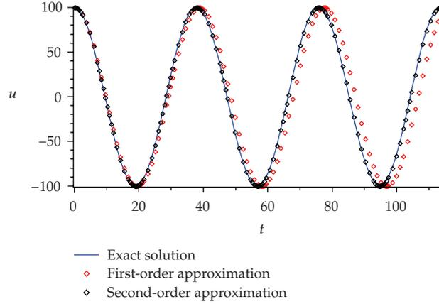
**Figure 6:** Comparison of approximate periodic solutions of Buckling of a Column equation (Case 1) with the exact one for  $m = 100.0$ ,  $l = 50.0$ ,  $P = 150.0$ ,  $k_1 = 70.0$ , and  $k_3 = 20.0$  with  $u(0) = 100.0$ .
