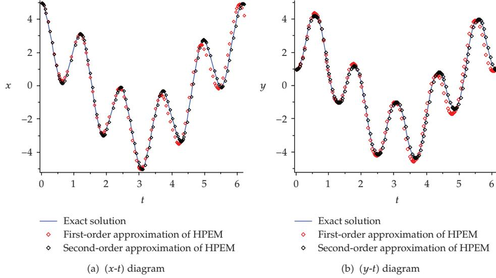
**Figure 7:** Comparison of the first- and second-order analytical approximate solutions with the exact solution for  $m = k_1 = k_2 = k_3 = 1.0$  with  $x(0) = 5.0$  and  $y(0) = 1.0$  (Case 2).
