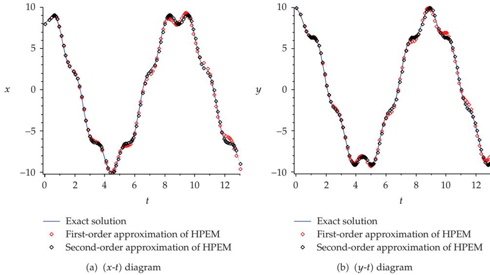
**Figure 8:** Comparison of the first- and second-order analytical approximate solutions with the exact solution for  $m = 2.0, k_1 = 1.0, k_2 = 3.0, k_3 = 5.0$  with  $x(0) = 8.0$  and  $y(0) = 10.0$  (Case 2).
