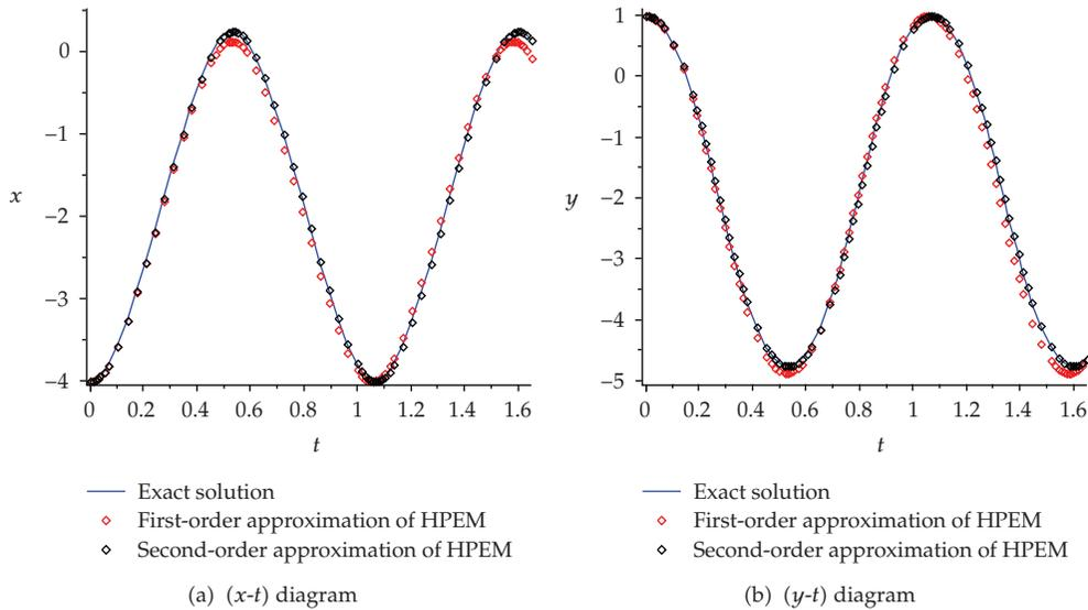
**Figure 9:** Comparison of the first- and second-order analytical approximate solutions with the exact solution for  $m_1 = 1.0, m_2 = 2.0, k_1 = 5.0, k_2 = 1.0$  with  $x(0) = -4.0$  and  $y(0) = 1.0$  (Case 3).
