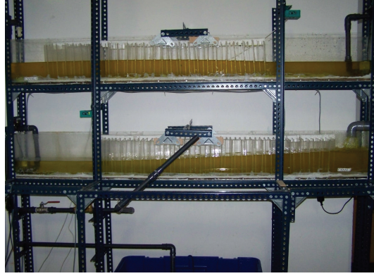
Figure 1: Frontal view of the experimental prototype canal.
