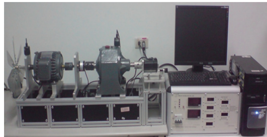
Figure 6: Actual hardware structure of the proposed fault diagnosis simulator.
