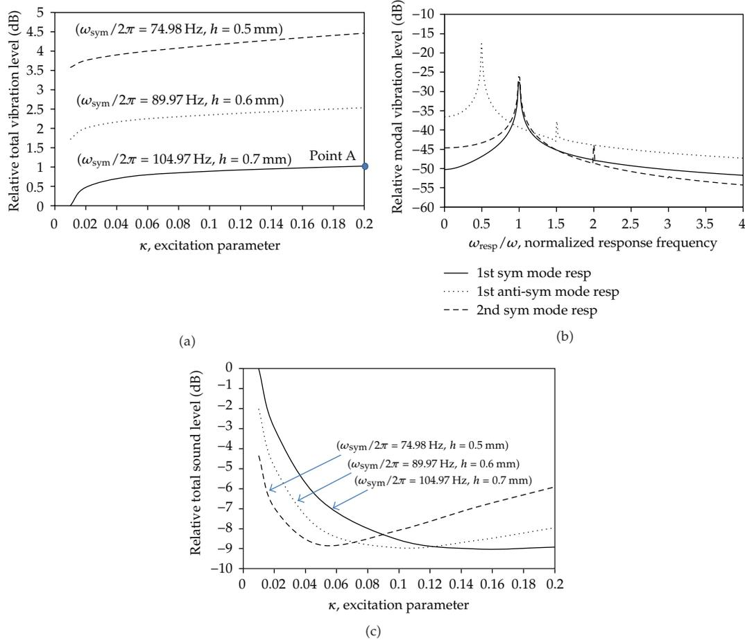
**Figure 3:** (a) Relative total vibration level ( $\omega_{sym}/\omega_{anti-sym} = 2, \omega = \omega_{sym}$ ), (b) relative modal vibration levels of point A in (a), (c) relative total sound level ( $\omega_{sym}/\omega_{anti} = 2, \omega = \omega_{sym}$ ).
