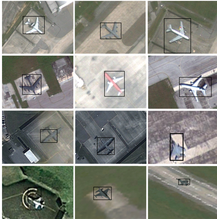
Figure 5: Examples of successful detections on satellite images and synthetic images. Note that simulation airplane models in the last two synthetic images are also correctly detected.
