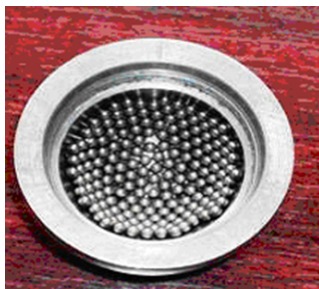
Figure 1: The MOM total hip prosthesis with rolling friction [11]
