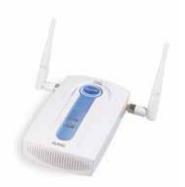
The secure and reliable ZyXEL B-3000 Intelligent Wireless LAN Access Point is a robust wireless LAN solution for Hot Spot and enterprise applications. The B-3000 can be easily integrated into an existing wired network to increase scalability and versatility as well as expand network connectivity.
