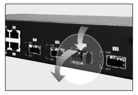
**2** Pull the transceiver out of the slot.
