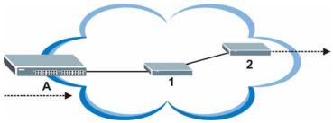
Switch A marks traffic flowing into the network based on the configured marking rules. Intermediary network devices 1 and 2 allocate network resources (such as bandwidth) by mapping the DSCP values and the associated policies.
