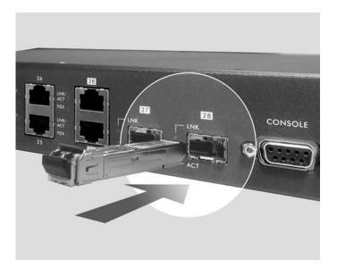
Figure 3-2 Transceiver Installation Example
