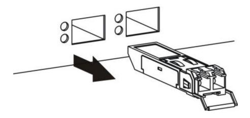
Figure 3-5 Transceiver Removal Example
