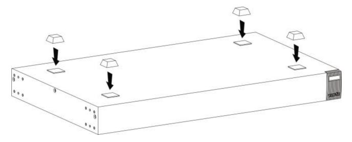
Figure 2-1 Attaching Rubber Feet
