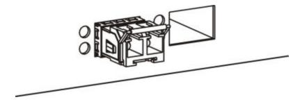
Figure 3-3 Installed Transceiver
