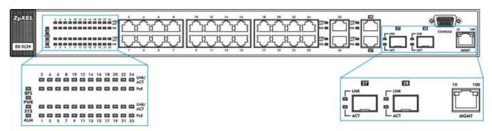
Figure 3-7 Front Panel LEDs
