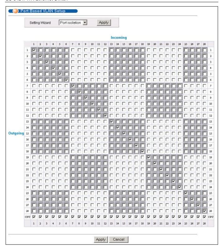
Figure 7-9 Port Based VLAN Setup (Port isolation)
