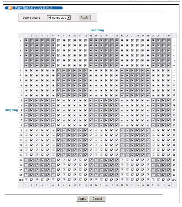
Figure 7-8 Port Based VLAN Setup (All Connected)
