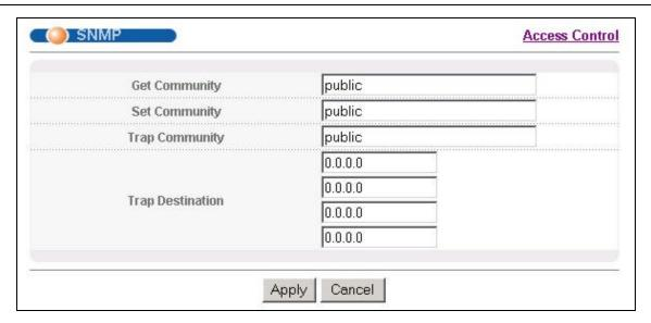
Figure 17-4 Access Control: SNMP
