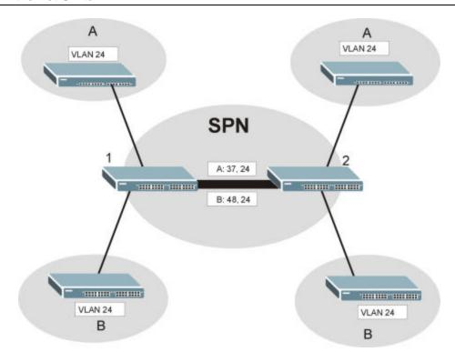
Figure 21-1 VLAN Stacking Example
