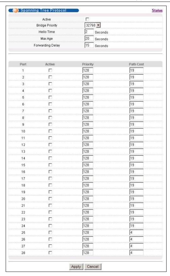
Figure 10-2 Spanning Tree Protocol: Configuring
