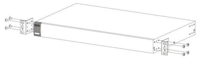
Figure 2-2 Attaching Mounting Brackets and Screws
