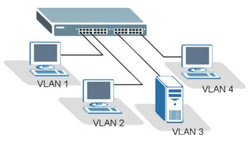
Figure 1-5 Shared Server Using VLAN Example
