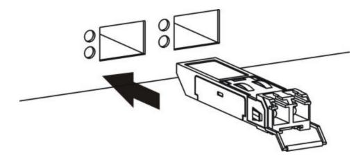
Figure 3-2 Transceiver Installation Example
