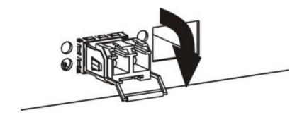
Figure 3-4 Opening the Transceiver's Latch Example
