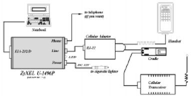
Fig. 14.1: Example 1 - U-1496P with a mobile phone
