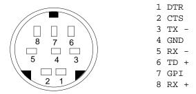
Fig. 23.1: Serial port of an Apple Macintosh
