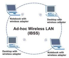
Figure 2-1 Ad-hoc Network Example
