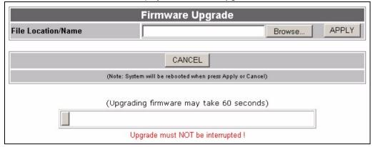
Specify the name of the firmware file in the **Local PC File Path** field or click **Browse** to locate the file and click **Apply** to start the file transfer process. The firmware must be a binary file and should have a .bin extension.
