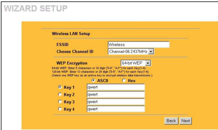
**ESSID** is a unique name to identify the ZyAIR in the wireless LAN. Enter a descriptive name.
