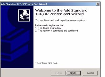
7 Enter the NPS-520's IP address in the **Printer Name or IP Address** field and click **Next**.
