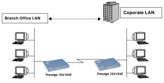
Figure 5-1. LAN-to-LAN Application with TCP/IP
