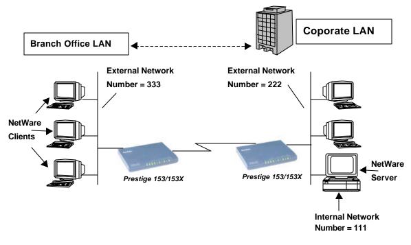
Figure 6-3. LAN-to-LAN Application with Novell IPX
