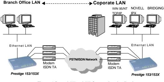
Figure 1-5. LAN-to-LAN Connection Application
