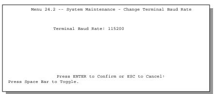
Figure 13-4. Menu 24.2 - System Maintenance - Change Terminal Baud Rate
