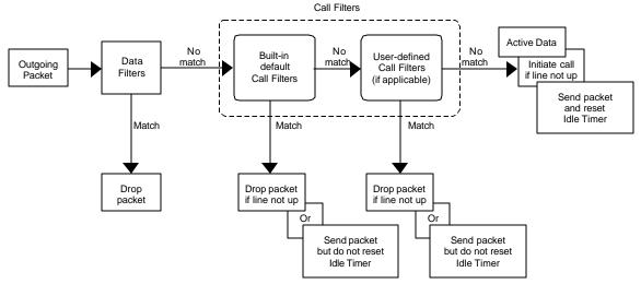
Figure 9-1. Outgoing Packet Filtering Process
