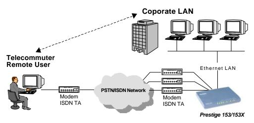
Figure 1-6. Telecommuting/Remote Access Application
