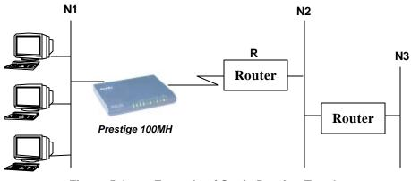
Figure 5-4. Example of Static Routing Topology
