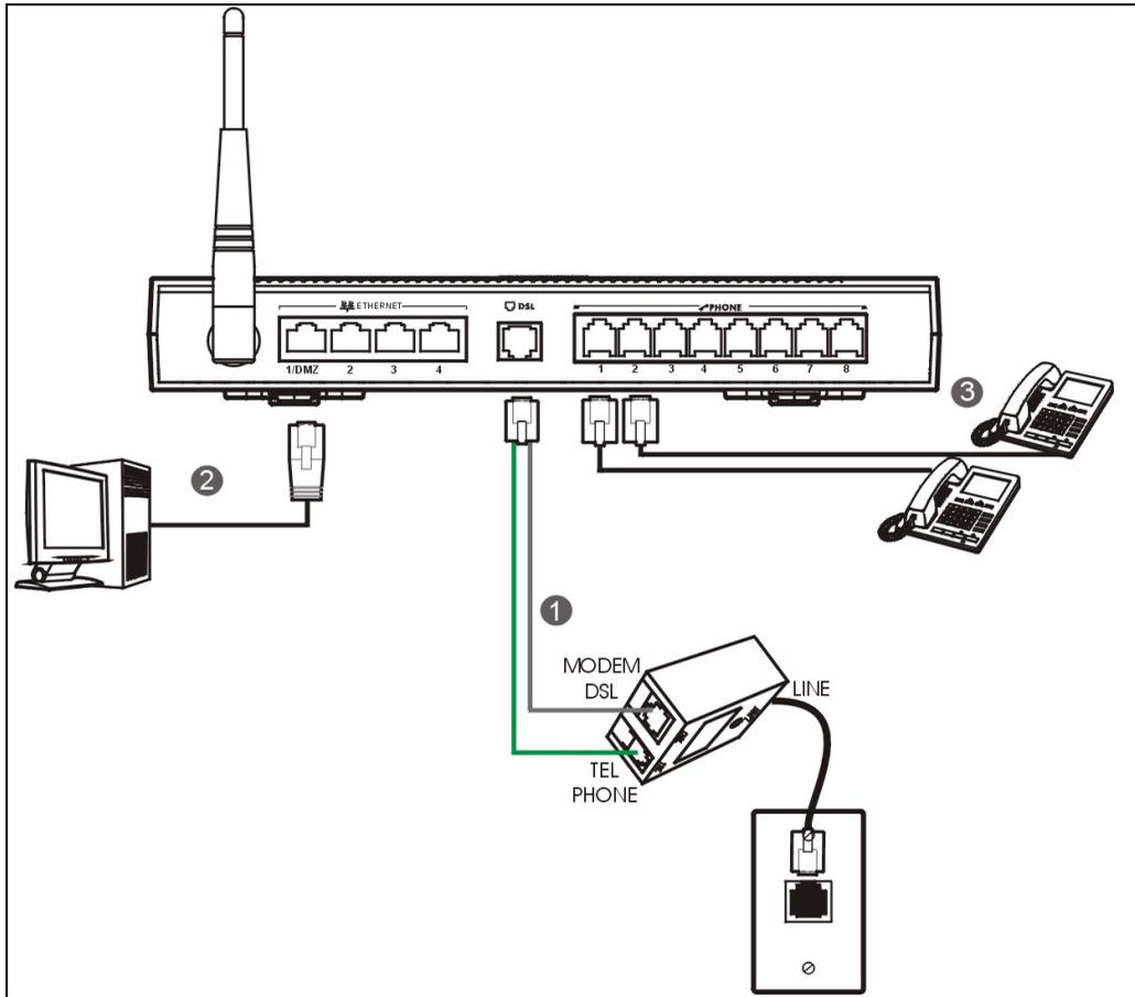
**1 DSL:** In the P-2608HWL-Dx, the **DSL** port handles both the ADSL and regular telephone service connections. Connect the v-shaped cable (with one gray and one green wire) to the P-2608HWL-Dx's **DSL** port. Connect the gray wire to the **MODEM or DSL** jack on a telephone or ISDN splitter (not included) and the green wire to the splitter's **TEL** or **PHONE** jack. Connect the **LINE** jack to your telephone wall outlet.
