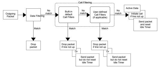
Figure 13-1 Outgoing Packet Filtering Process
