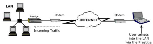
Figure 19-1 Telnet Configuration on a TCP/IP Network
