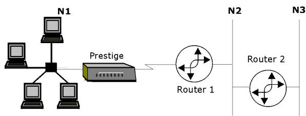
Figure 10-1 Example of Static Routing Topology
