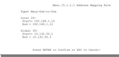
Figure 11-23 Example 4: Menu 15.1.1.1 — Address Mapping Rule
