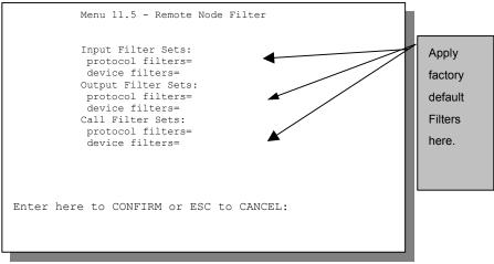
Figure 13-15 Filtering Remote Node Traffic
