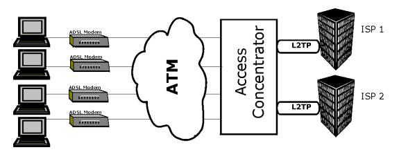
Diagram 1 Single-PC per Modem Hardware Configuration
