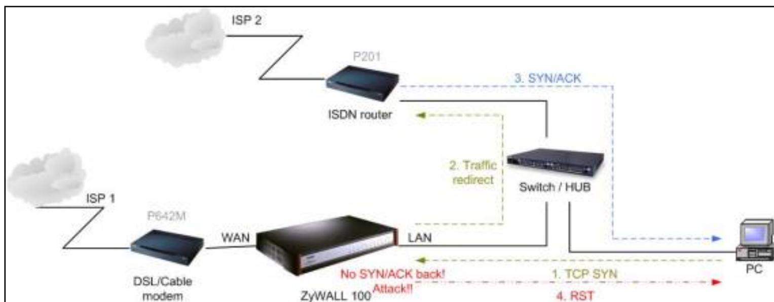
The above figure indicates the "**triangle route**" topology. It works fine if you turn off firewall function on P334WT box. By default, your connection will be blocked by firewall because of the following reason.
