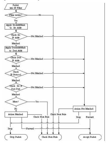
Figure 198 Executing an IP Filter
