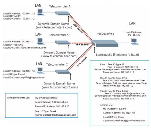
Figure 92 Telecommuters Using Unique VPN Rules Example
