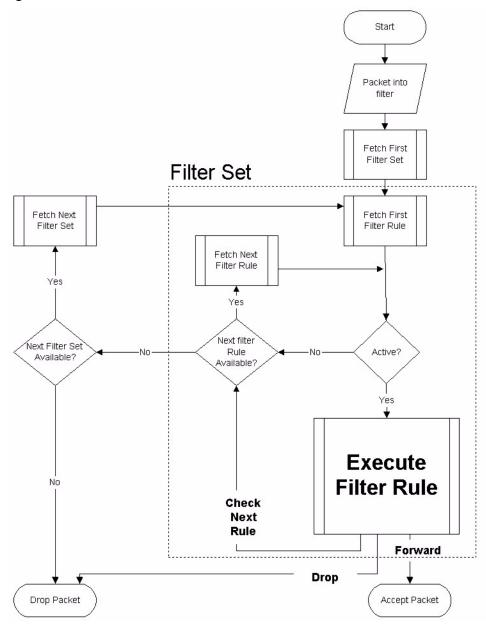
Figure 194 Filter Rule Process
