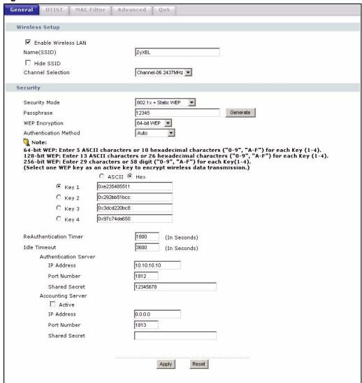
Figure 41 Wireless: 802.1x and Static WEP
