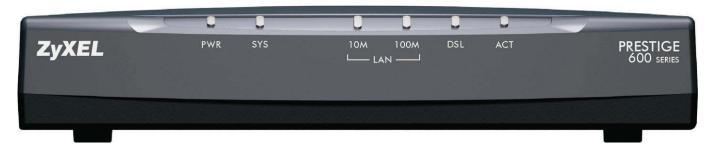
The **Power** LED turns on, the **SYS** LED blinks and turns steady on. The **SYS** LED turns red if power is too low. The **LAN** and **DSL** LEDs turn on, if they are properly connected.
