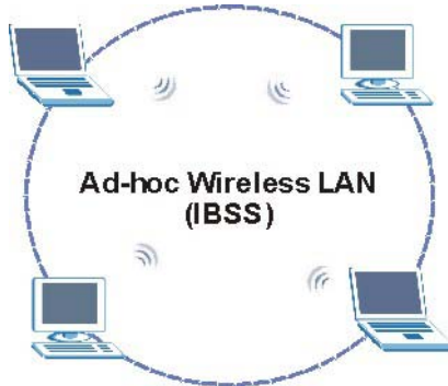
Diagram C-1 Peer-to-Peer Communication in an Ad-hoc Network
