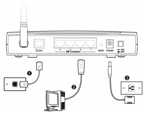
1 DSL: Use a telephone wire to connect your P-660HW-D's DSL port to a telephone jack (or to a splitter, if one is already installed).
