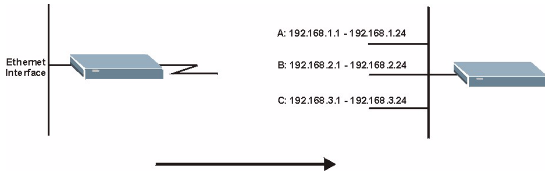
Figure 52 Physical Network & Partitioned Logical Networks
