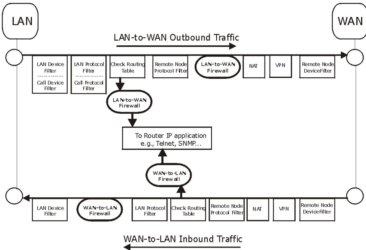
Diagram 3-1 Big Picture— Filtering, Firewall, VPN and NAT
