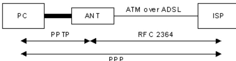
Diagram 7-1 Transport PPP frames over Ethernet
