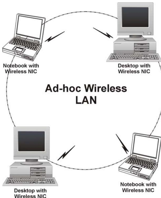
**Diagram 4-1 Peer-to-Peer Communication in an Ad-hoc Network**
