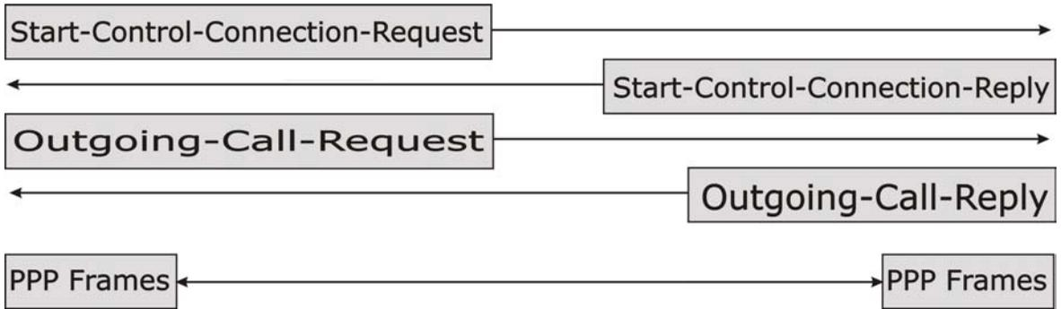
**Diagram 7-3 Example Message Exchange between PC and an ANT**
