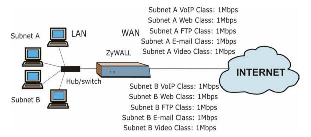
Figure 18-3 Application and Subnet-based Bandwidth Management Example
