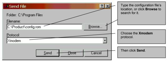
Figure 21-8 Example Xmodem Upload
