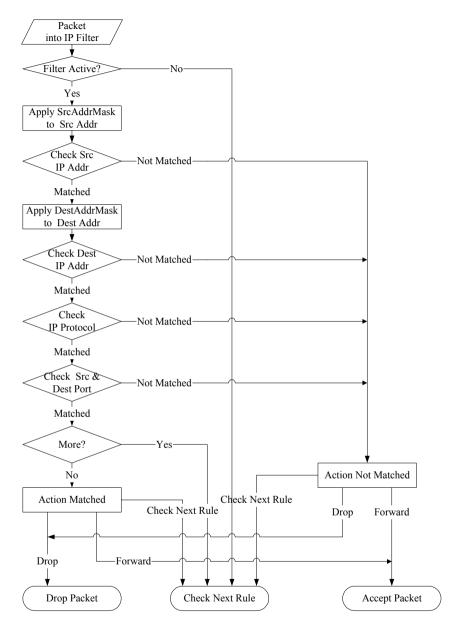
Figure 31-7 Executing an IP Filter
