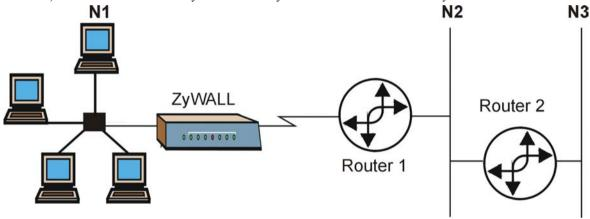
Figure 10-1 Example of Static Routing Topology
