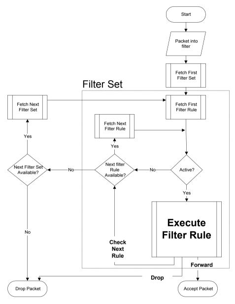
Figure 31-2 Filter Rule Process
