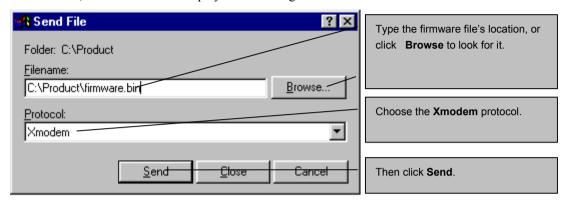
Figure 34-17 Example Xmodem Upload
