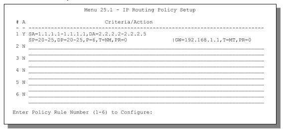
Figure 37-4 Menu 25.1: Sample IP Routing Policy Setup
