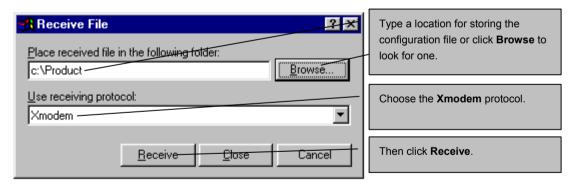
Figure 34-5 Backup Configuration Example
