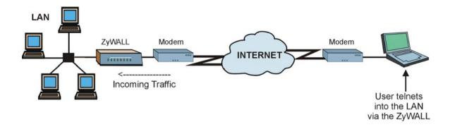
Figure 16-1 Telnet Configuration on a TCP/IP Network
