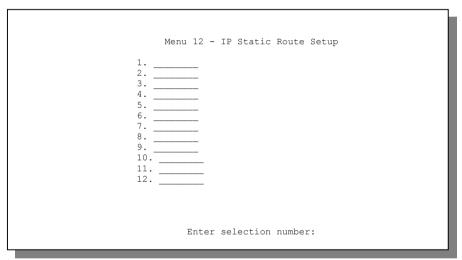
Figure 28-1 Menu 12: IP Static Route Setup (ZyWALL 10W)
