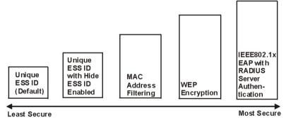
Figure 6-2 ZyWALL Wireless Security Levels
