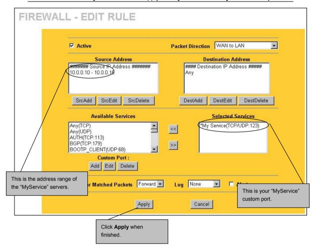
Figure 12-10 MyService Rule Configuration (ZyWALL100)
