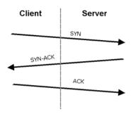
Figure 11-2 Three-Way Handshake
