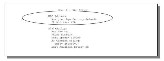
Figure 23-1 MAC Address Cloning in WAN Setup
