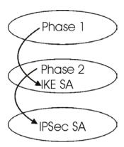
Figure 15-5 Two Phases to Set Up the IPSec SA
