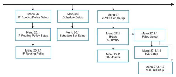
Figure 21-6 Schedule Setup and IPSec VPN Configuration SMT Menus
