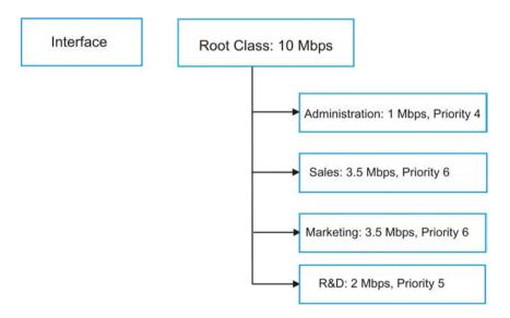
Figure 18-5 Maximize Bandwidth Usage Example
