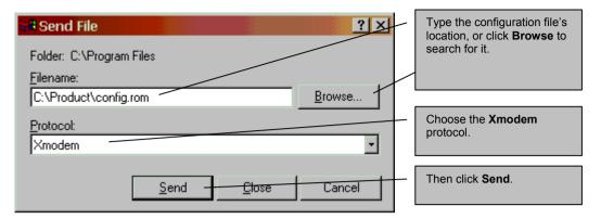
Figure 2-2 Example Xmodem Upload
