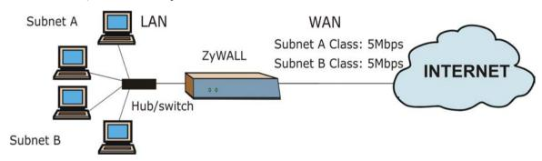
Figure 18-2 Subnet-based Bandwidth Management Example
