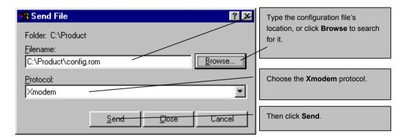
Figure 34-19 Example Xmodem Upload
