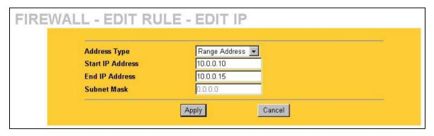
Figure 12-8 Firewall Rule Edit IP Example
