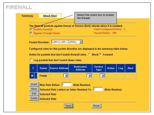
Figure 12-3 Enabling the Firewall (ZyWALL 100)
