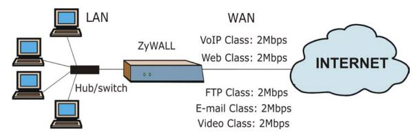
Figure 18-1 Application-based Bandwidth Management Example
