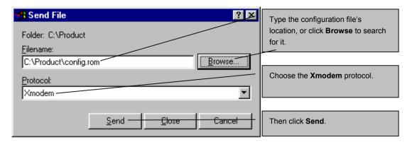
Figure 34-11 Restore Configuration Example
