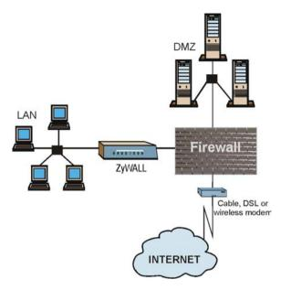
Figure 1-1 Secure Internet Access via Cable, DSL or Wireless Modem
