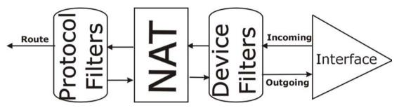
Figure 31-12 Protocol and Device Filter Sets
