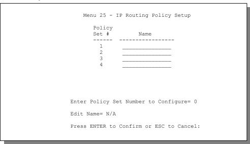
Figure 37-1 IP Routing Policy Setup
