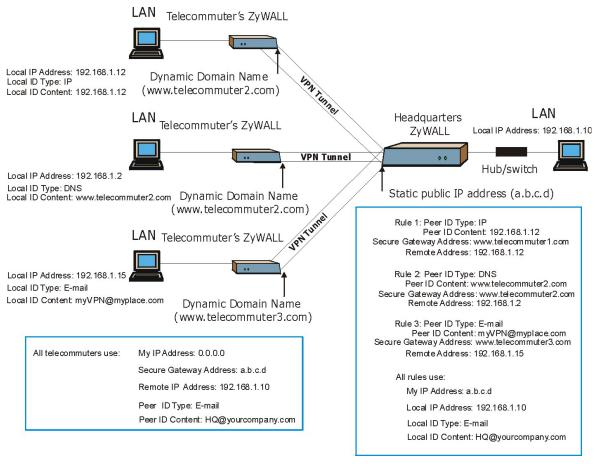
Figure 15-11 Telecommuters Using Unique VPN Rules Example
