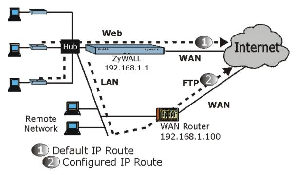
Figure 37-7 Example of IP Policy Routing
