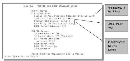
Figure 24-4 Menu 3.2: TCP/IP and DHCP Ethernet Setup
