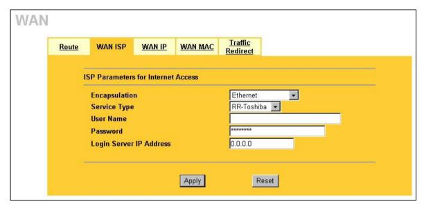
Figure 8-2 Ethernet Encapsulation
