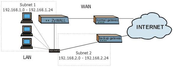
Figure 8-9 Traffic Redirect LAN Setup
