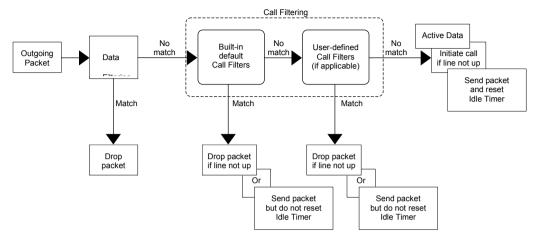
Figure 31-1 Outgoing Packet Filtering Process
