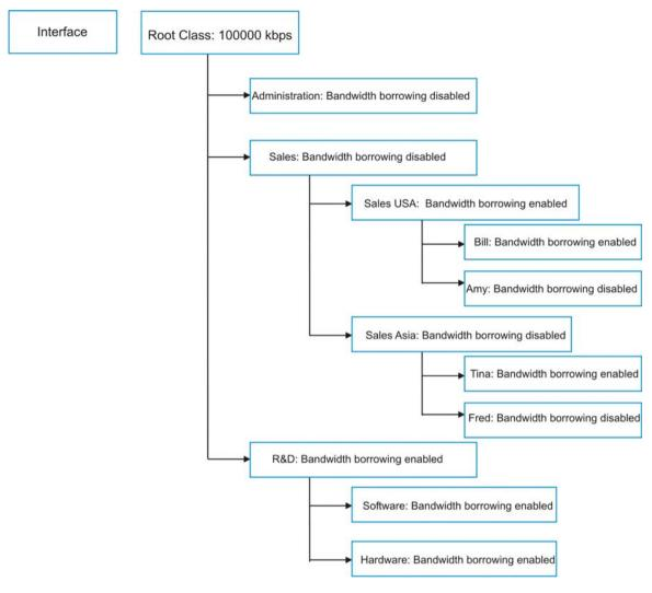
Figure 18-6 Bandwidth Borrowing Example
