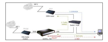
The above figure indicates the "**triangle route**" topology. It works fine if you turn off firewall function on ZyWALL box. However, if you turn on firewall, your connection will be blocked by firewall because of the following reason.
