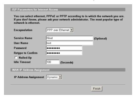
Select "**Dynamic**" if the ISP provides the IP dynamically, otherwise select "**Static**" and enter the static IP given by ISP in the "**IP Address**" field.
