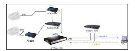
(C) To resolve this conflict, we add an option for users to allow/disallow such **Triangle Route** topology in both CI command and Web configurator. You can issue this command, "**sys firewall ignore triangle all on**", to allow firewall bypass triangle route checking. In Web GUI, you can find this option in firewall setup page.
