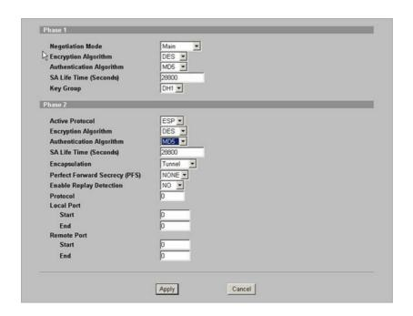
Step 4. Using Certificate in VPN on ZyWALL P1
