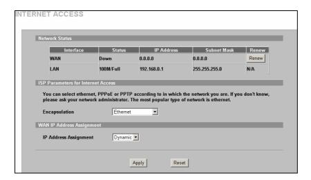
Select Encapsulation type according to your environment. Ex. If you are in a hotel, most likely you would use Ethernet with Dynamic IP address assignment
