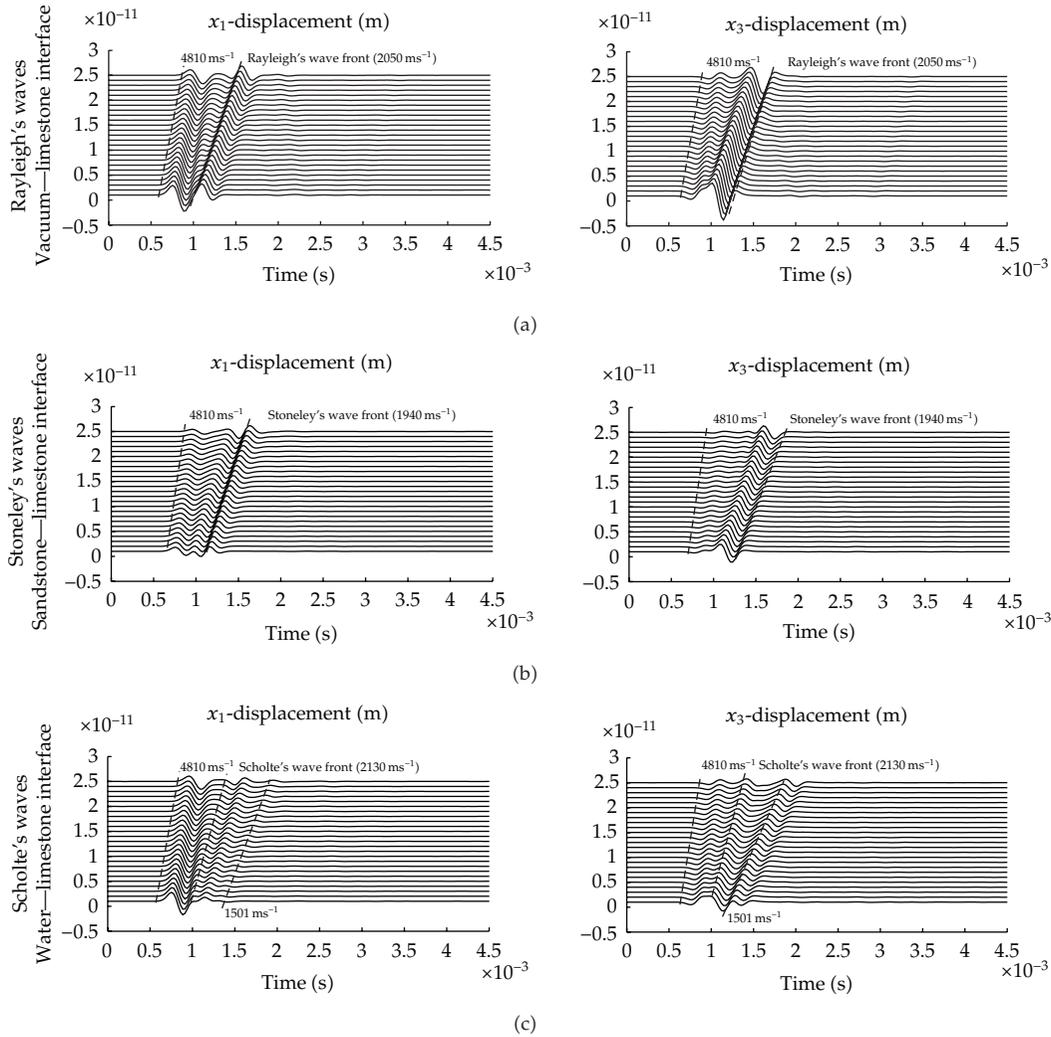
**Figure 5:** Synthetic seismograms for three different interfaces. (a) Vacuum-solid interface, (b) solid-solid interface, and (c) fluid-solid interface.  $x_1$  (left) and  $x_3$  (right) components of displacement are plotted. Materials 2 from the Table 1 are used for the analysis.
