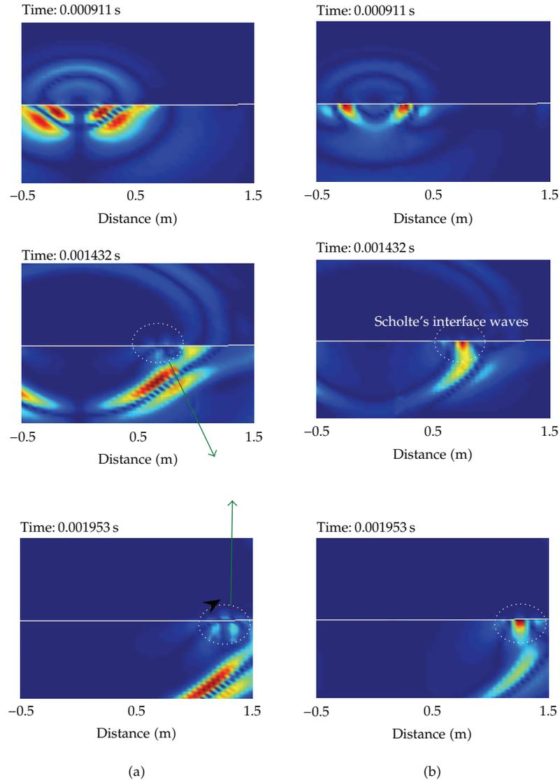
**Figure 6:** Snapshots by IBEM for the complete 2D water-sandstone interface model are shown. A grid of  $51 \times 51$  receivers, spaced using a distance increment of 0.04 m, is required. Column (a) plots the results of pressures in the fluid and displacements in the  $x_1$  direction for the solid, while the column (b) plots pressures in the fluid and displacements in the  $x_3$  direction for the solid.
