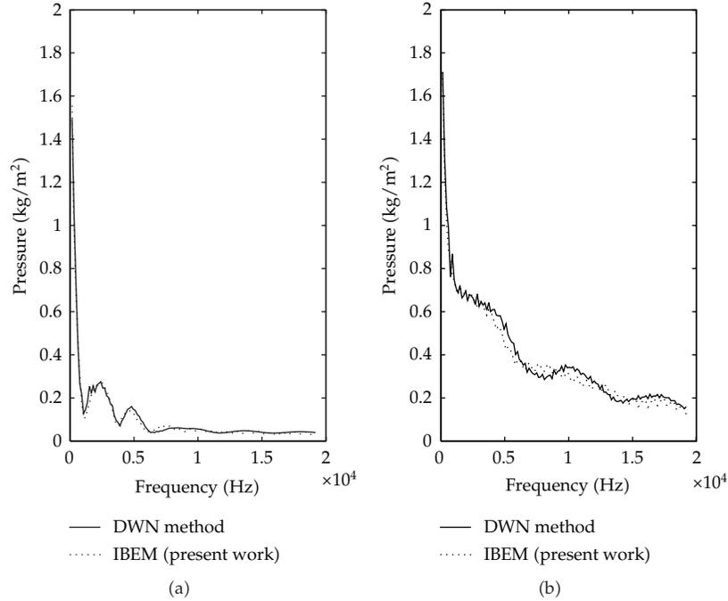
**Figure 7:** Spectra of pressures for water-sandstone (left) and water-limestone (right) interfaces. Results obtained by IBEM are plotted using dotted lines, while those obtained by means of DWN are drawn with continuous lines. Good agreement between IBEM and DWN is observed.
