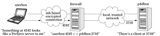
Packets ultimately destined for your client's port 4242 are first sent to the firewall, and ssh forwards them securely to your client. Likewise, connections made to port 4242 of the firewall machine will end up being routed to port 3710 of the Perforce server.
