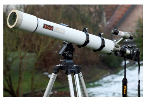
A Vixen 80M refracting telescope with a Nikon D80 and a solar filter attached. A small astronomical telescope like this can be used with most DSLRs and is much cheaper than a super-telephoto lens.
