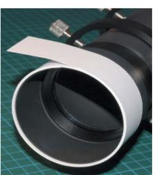
Taping the filter foil to a cardboard ring
