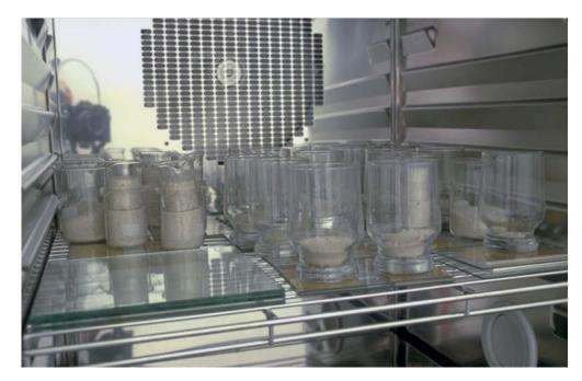
A climate-controlled chamber is one of the more important (and expensive) tools for artificially aging test samples at high temperatures and predefined humidity levels. The Arrhenius equation is then used to analyze the results and provide an estimate of the lifespan of the tested material at room temperature.
