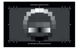
An opto-electronic conversion function (OECF) is used to determine a digital camera's ability to convert brightness values into digital image data. We use a standardized OECF chart and an integrating sphere (also known as an Ulbricht sphere) to reliably determine each camera's noise behavior and dynamic range.
