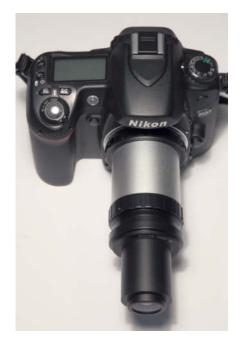
A Zeiss Abbe Barlow lens attached to a Nikon D80 using a T2 adapter. You can use a lens like this and extension tubes to extend focal length as far as you like.
