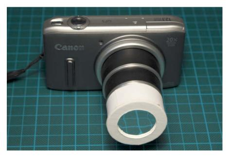
A Canon compact fitted with a home-made solar filter. The camera's  $20\times$  optical zoom is powerful enough to make large sunspots visible.
