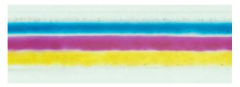
Because the colors in analog film and photo paper age at different rates, both media develop various colored casts over time. The process can be slowed down, but not completely stopped, by storing affected material at low temperatures. This image shows a cross-section of a slide film viewed through a microscope.
