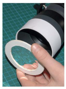
Fixing the filter to the tube
