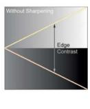
The sharpening curves show how markedly the contrast in the first three rows of pixels on either side of an edge is increased. The red curve is the closest to the edge and is altered the most. The green curve represents the second row and the blue curve the third, which in this case remains unchanged. Curves that meet and follow the top and bottom horizontal axes indicate oversharpening, which becomes visible in real-world images in the form of light or dark sharpening artifacts.
