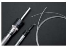
Optical fibers, available in various widths, are ideal for creating fine lines and patterns. You can combine several to create interesting visual effects. A piece of thin aluminum tubing is another way to focus the light from a lamp.
