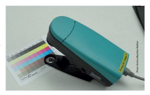
Measure, measure and measure again. Here, a non-laminated reference color sample is scanned at the University of the Arts in Bern, Switzerland. The university conducted three large-scale tests to examine how Diasec face-mounting affects the lifespan of analog and digital prints.
