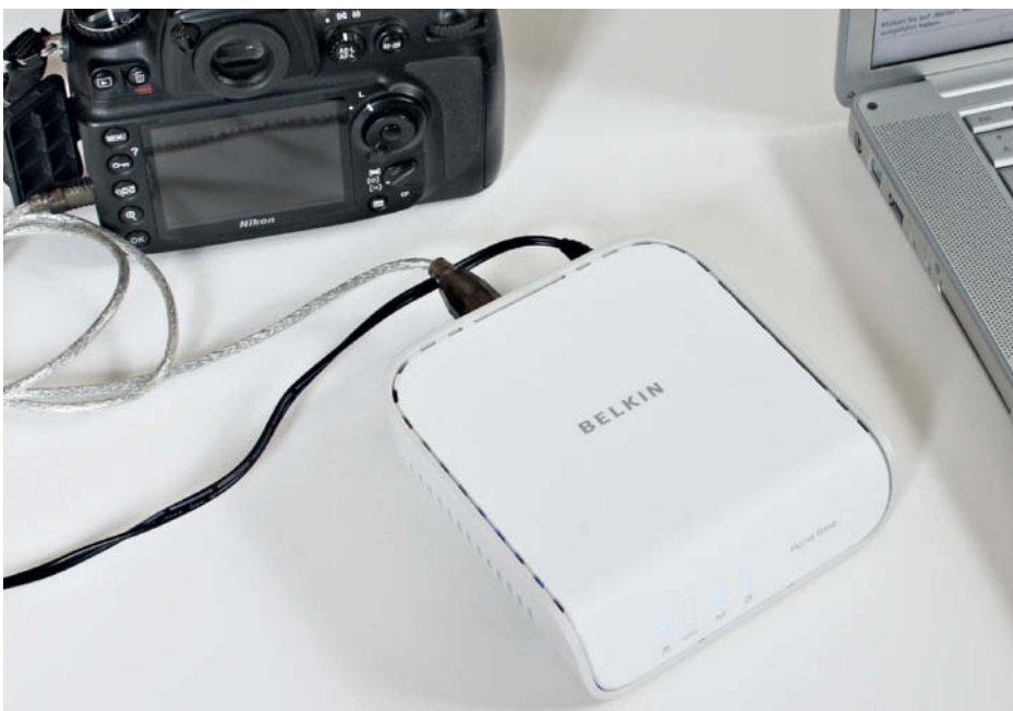
This is what the "wireless" configuration using the Belkin "Home Base" USB WLAN adapter looks like in practice. Here, too, an outlet is required to supply power to the adapter.
