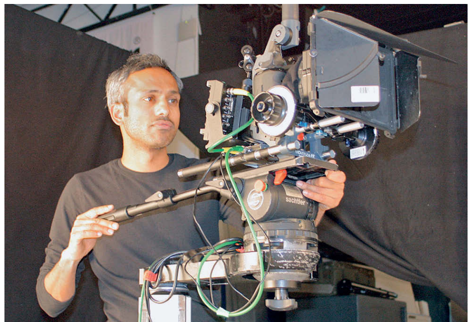
The white ring around the focus knob makes it easier for the focus puller to mark the start and end positions for each shot.
