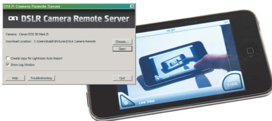
DSLR Camera Remote saves all images on the host computer. The Live View and preview pictures are transferred to the iPod Touch.
