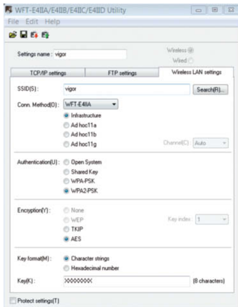
The add-on program WFT Utility allows you to configure the network settings for the WFT-E4 II on the computer and transfer them via USB cable or memory card to the Canon camera
