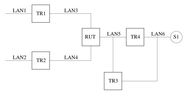
Figure 4.6: Sending (\*,G) Join/Prune Messages test setup
