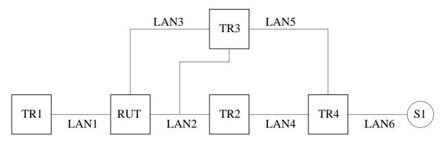
Figure 5.1: (S,G) Assert message state machine test setup
