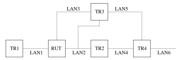
Figure 6.6: Receiving and using the RP-Set test setup
