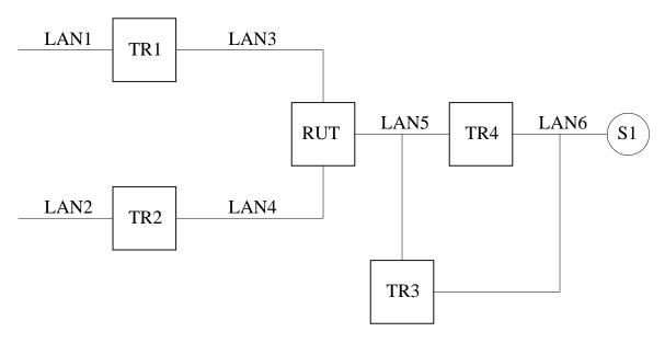
Figure 4.5: Sending (\*,\*,RP) Join/Prune Messages test setup
