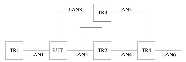
Figure 6.2: Non-candidate BSR state machine test setup
