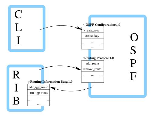
Figure 1: Example XRL Targets and clients: OSPF, RIB, and CLI. OSPF and RIB processes are XRL targets. OSPF supports XRL interfaces "OSPF Configuration/1.0" and "Routing Protocol/1.0": the CLI is a client of the "OSPF Configuration/1.0" interface and the RIB a client of the "Routing Protocol/1.0" interface. RIB supports XRL interface "Routing Information Base/1.0": the OSPF is a client of that interface.
