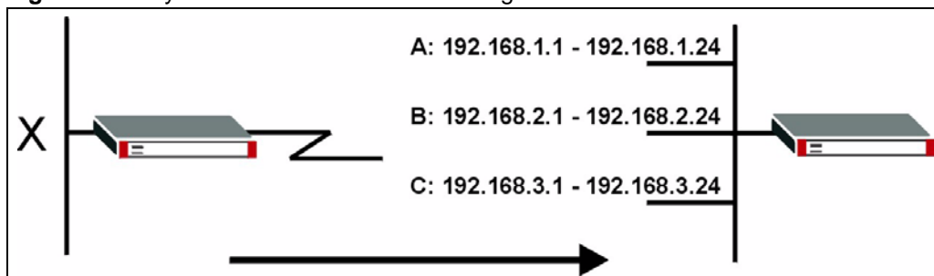
Figure 54 Physical Network & Partitioned Logical Networks
